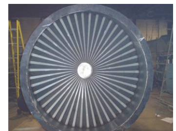
Internal view of the QUENCHER cell
