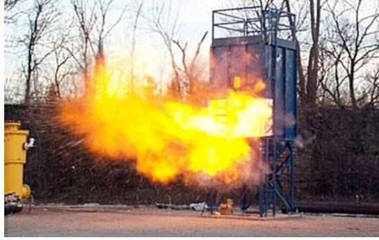
Fire and Explosion in Dust Collector
